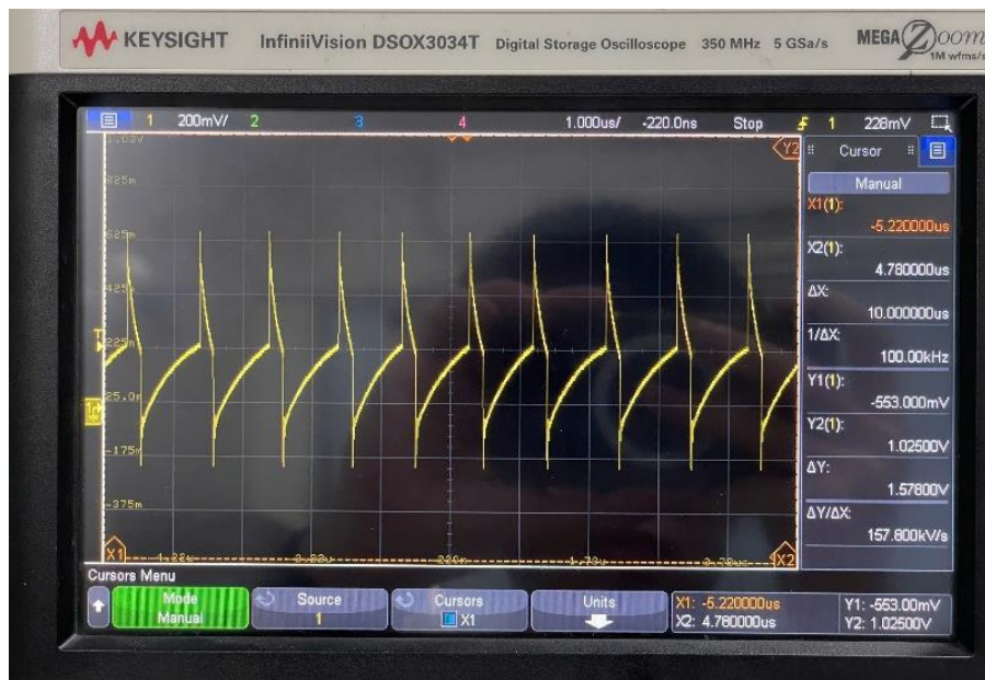
Figure 14. The output signal of the block produces a random oscillation signal.
