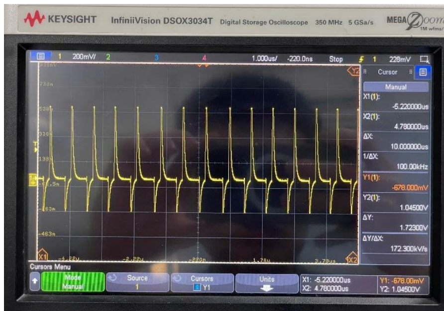
Figure 16. The output signal of the block produces a narrow pulse signal.
