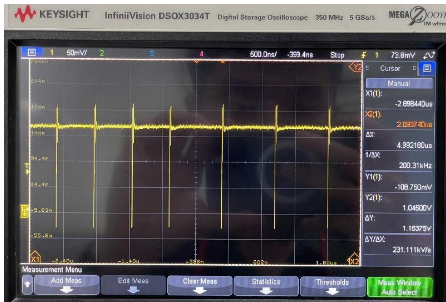
Figure 17. Output signal results in an ultra-narrow pulse generator and amplifier
